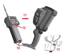
Caution: Use only finger pressure to remove or attach tips. Using force (including pliers or other tools) might damage the bending neck. Take care not to cross the threads. To reduce cross-threading risk: When installing a tip by hand (6.1mm & 8.4mm) or with an installation tool (4mm), rotate the tip counter clockwise to level the threads before rotating clockwise to thread the tip on the camera. Reverse the leveling process when removing tips.
