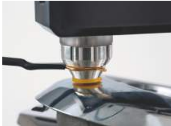
STEP Test measuring cell placed on a specimen
