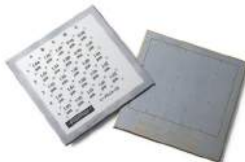
Standards for calibrating the measurement system with 5 x 5 individually-measured test areas
