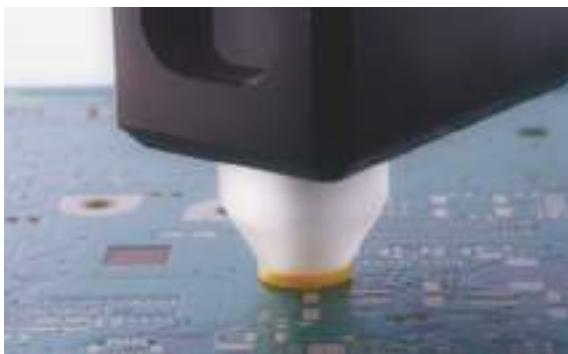
Measuring the thickness of remaining tin on a printed circuit board
