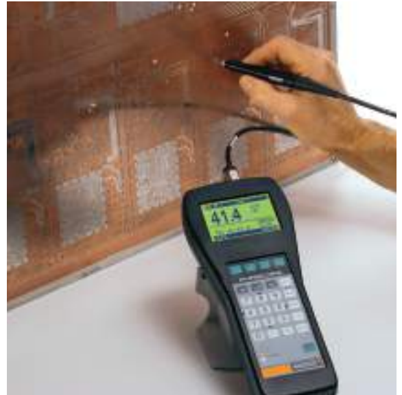
Measuring copper thickness in through-holes using the ESL080B probe
