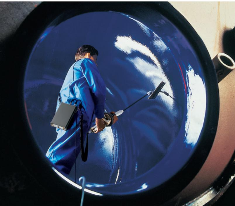
Pore testing of the enamel coating of a boiler, using the POROSCOPE®
