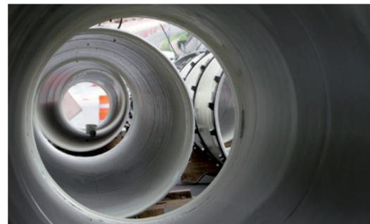
Testing the interior coating of pipes during pipe manufacturing
