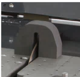
Mode: Metallographic cutting of small samples
