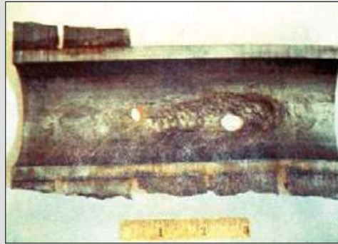
Localized corrosion damage in carbon steel can be confirmed using visual methods
