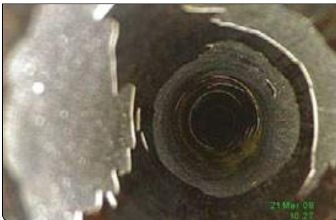
Air fin heat exchanger tube damage can cause significant operational problems
