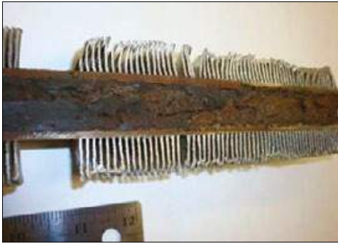
Air fin heat exchanger tube damage can cause significant operational problems
