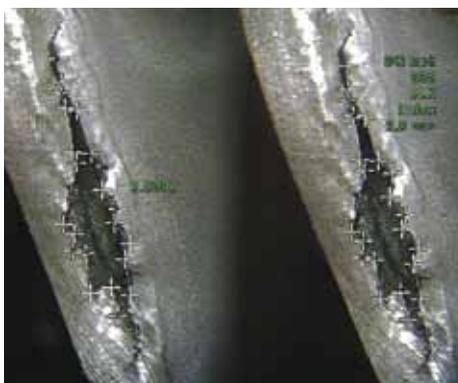
StereoProbe® area measurement screen shot from XLG3 VideoProbe
