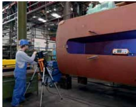
Inspection of ship assemblies using industrial X-ray
