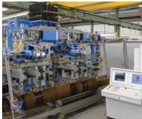
SNUP ultrasonic pipe testing system
