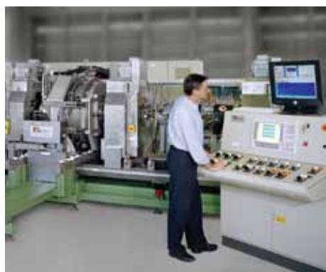
ROTA ultrasonic bar, tube and pipe testing system
