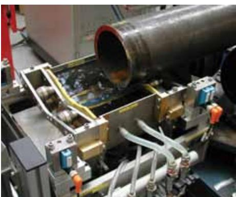
GRP ultrasonic tube and pipe testing system
