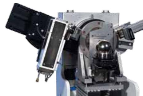
XRD stress analyser with Meteor1D detector
