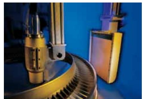
Detector array installed in a testing machine
