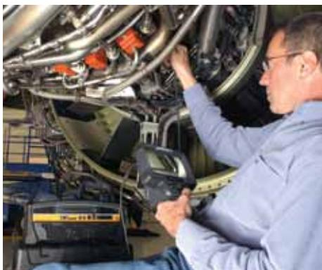
Aircraft engine inspection using the XLG3™ VideoProbe
