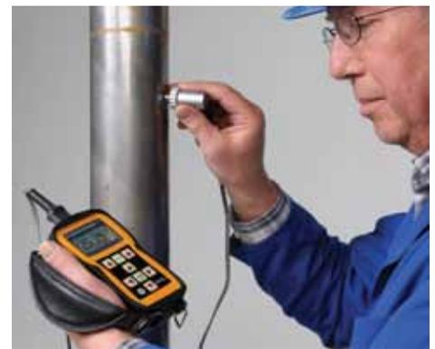
DM5E ultrasonic thickness gaging of pipes
