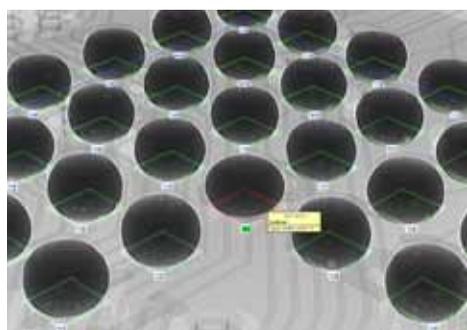
2D X-ray inspection: open BGA joint
