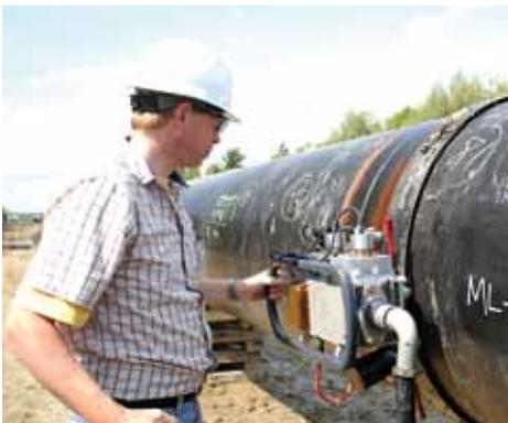
Weldstar mobile ultrasonic inspection system
