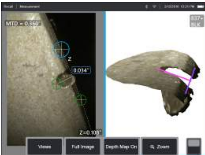
Conventional Measurement on a Diagonal
