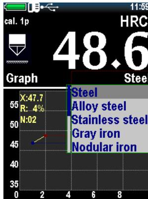
During the measurement you can select other hardness scale. The displayed measurement reading will be converted according with the new hardness scale if it is calibrated.
