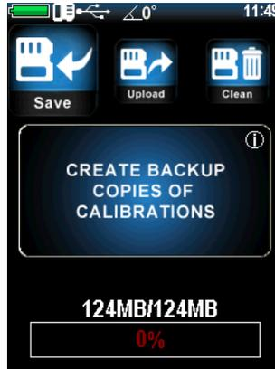
After calibration of the probe is recommended to create a backup copy of the calibration (usually the manufacturer makes the calibration of 1-2 scales, to check the probe). This is done in order to be able to resume adequate calibration after incorrect settings in the future.
