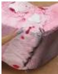
Visible penetrant crack indication on D-70
