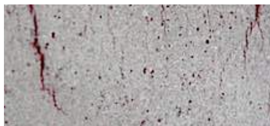
High temperature penetrant VP-302 crack indication on D-702 developer film.
