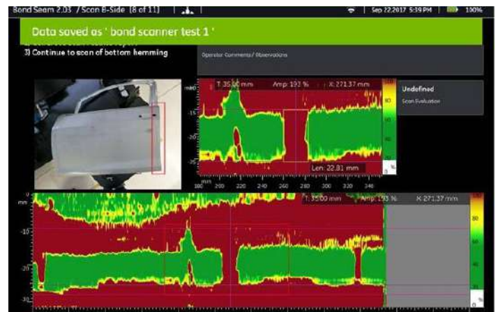
Green indicates strong adhesive bonding; Red indicates missing adhesive Note areas of slight adhesive leakage
