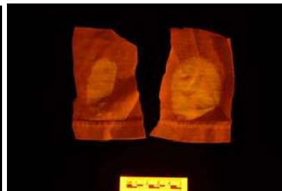
Fig. 11. Honey (left) and chlorine bleach (right) on cloth, illuminated by 450nm and viewed through orange goggles.
