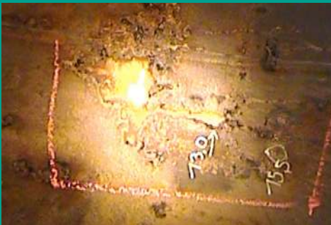
Visual confirmation of corrosion on the ID surface of the vessel.
