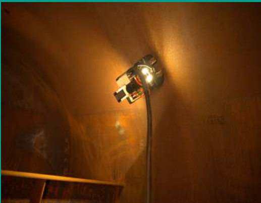
3D-structured light for detailed mapping inside a vessel.
